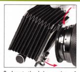
Insert the brim section of the adapter ring into the adapter ring groove on the rear mount board. Then, place the rear mount board flush against the adapter ring. Finally, fix securely with the adapter ring fixing knob. Of course, the rails should be oriented on the side of the camera base, when attached in this manner.
